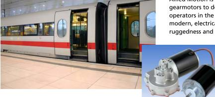
Allied's brush and brushless DC motors and gearmotors are cost-effective, yet offer the durability required by door system designers. They are also prized for their high performance and compact size, making them especially suited for use in space-restricted door system applications.
