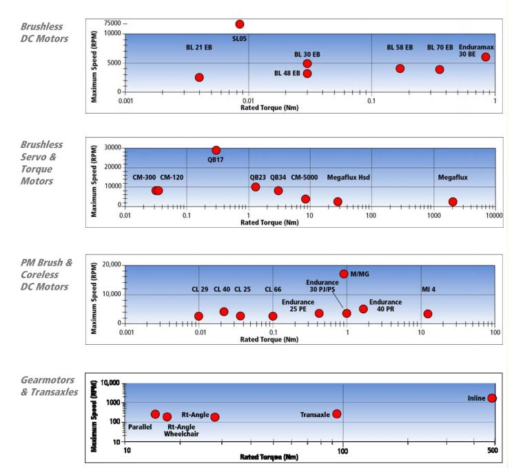
\* Charts indicate maximum speed and maximum rated torque points for each motor or motor series.
